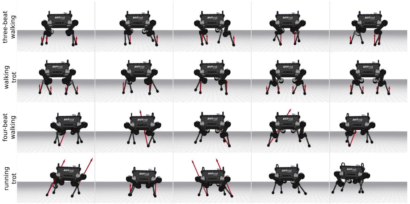
Fig. 9: Snapshots of different computed gaits: three-beat walking, walking trot, four-beat walking and running trot. Red arrows represent contact force vectors.
